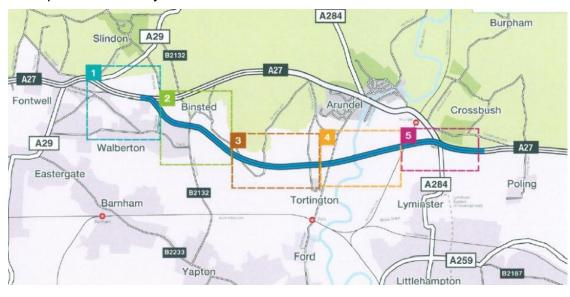
The Grey route is shown above and is an 'off-line' solution. It runs from the existing Crossbush Junction, in the east (although the junction will be remodelled), over the railway line, crossing the River Arun and its flood plain on a viaduct. It then passes to the south of Binsted Wood, through part of the Avisford Golf Course, crossing Tye Lane, to reconnect with the existing A27 around Copse Lane, Walberton.
